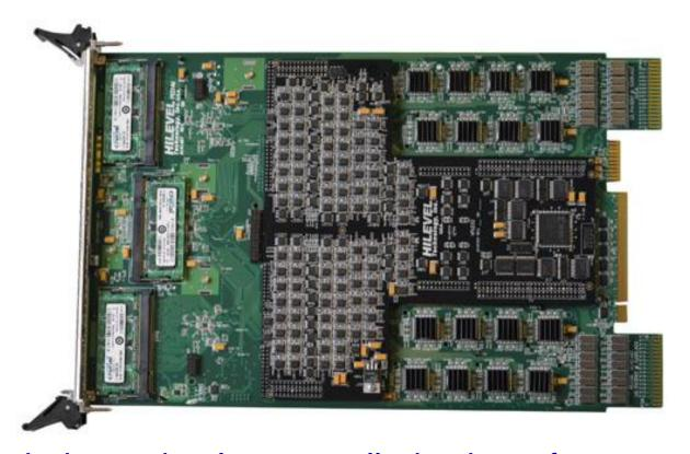
32 independently controlled pins; format control, timing select; drivers, receivers, PMU/32, 1A DUT Power, programmable loads, 5mV resolution
