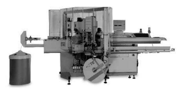
The Alpha 356 fully automatic crimping machine has room for up to seven processing stations.
