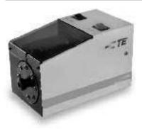
The AT-ST machine strips and twists wires with sizes from  $0.03~\text{mm}^2$  up to  $6~\text{mm}^2$  / AWG 32-10. The adjustable turret head with 8 guide tubes for different wire sizes centralizes positioning of wires. Special ground blades cut and strip special insulations
