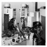
The Gamma 333 PC-B lead maker is a flexible fully automatic crimping machine for efficient wire processing. It processes cross sections in a range from 0.13-5.0 mm<sup>2</sup> (AWG 26-AWG 10).
